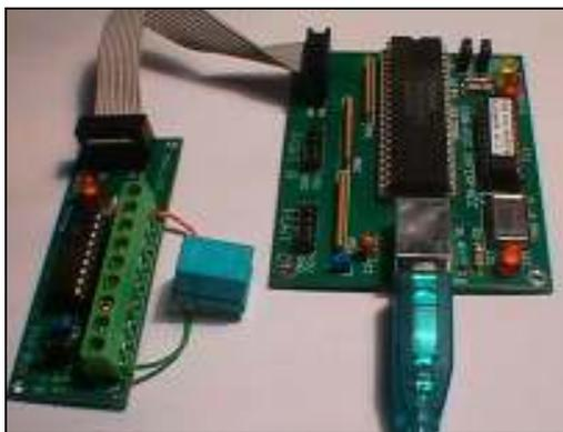
Figure 11. A Relay/Stepper Motor Interface connected to the USB PIO Card (via ribbon cable).
