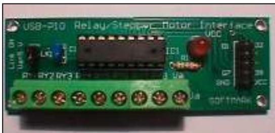
Figure 10. A Relay/Stepper Motor Card Interface.
