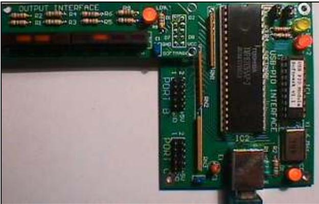
Figure 8. LED Interface connected to port A (direct connection to the USB PIO Card).
